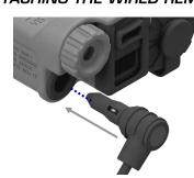
TO ATTACH: INSERT REMOTE CONNECTOR INTO REMOTE CONNECTOR PORT AND PRESS UNTIL IT CLICKS.
