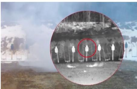
ENVG-B provides targeting and identification in all battlefield conditions as well as light levels including degraded visual environments such as smoke, fog and debris. The goggle includes L3Harris' high-performance white phosphor image intensification technology fused with thermal imagery; thereby bridging the gap in performance and capability for both of these sensors.
