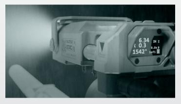
The integrated ballistic computer measures temperature, pressure, humidity, inclination, cant and heading. In addition, wind speed and direction may be entered manually or via Bluetooth to calculate a ballistic solution. These capabilities make the RAPTAR Xe optimal for precision small arms engagements in all environments providing illumination and accurate targeting out to 1800m [1500m on 10% reflective man-sized target, 2000m on 30% reflective man-sized target].
